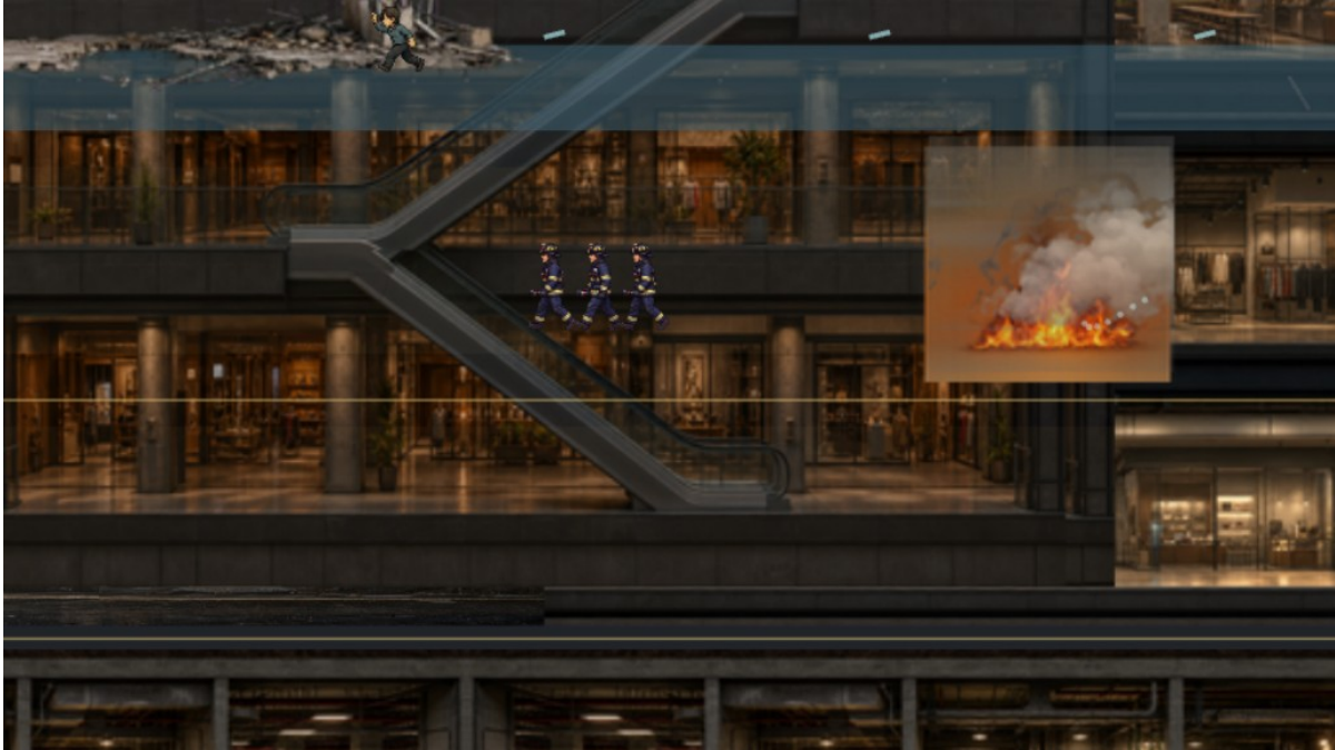
Figure 2 - Firefighters travel horizontally through the escalator area instead of following its slope.
